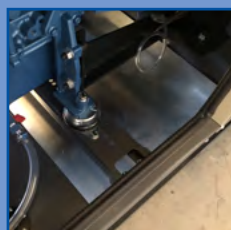
Bundled base environmentally friendly - to contain the liquids in the event of a spill
