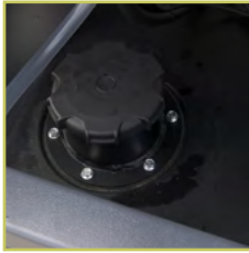
Tank filler wide tank refilling point
